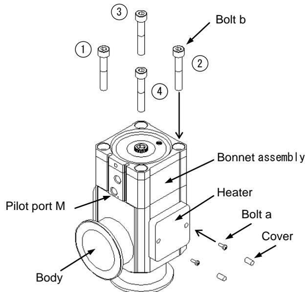
Apply 0.2MPa of air pressure to the pilot port M (for main pumping). Tighten bolt b in numerical order to assemble the body and the bonnet assembly. When tightening bolt b, tighten manually until the O ring is compressed, then perform extra tightening in diagonal order. For models with heater, tighten bolt a to mount the heater to the body. Insert the cover.
