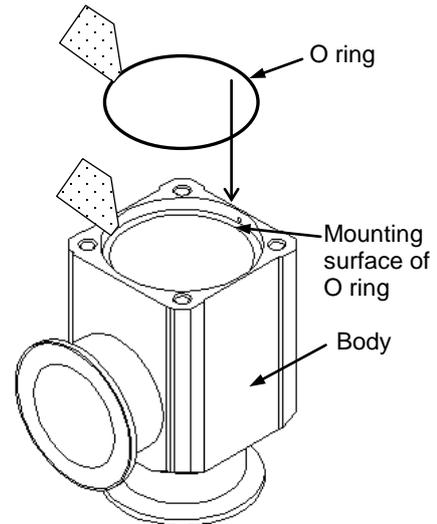
Wipe off the dust from the external seal O ring surface and the mounting surface of the body O ring. Place the O ring on the O ring mounting surface.
