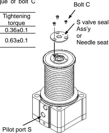
Apply 0.3MPa of air pressure to the pilot port S. Place the needle seat or S valve seal assembly, and tighten bolt c to fix them. When tightening bolt c, first tighten manually until the O ring is compressed, then perform extra tightening.
