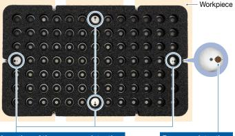
Location of the pressure detection port in of a foam hole (4 locations)
