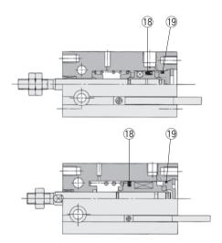
\* The numbers are the same as the "Construction" of the Best Pneumatics No.2 Series CU.
