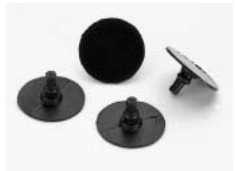
Normal elastomers and printing inks can sometimes combine to cause swell and hence distortions in the printing industry. So we investigated.
