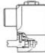
OPTION Y – MANUAL OVERRIDE – VALVE MAY BE OPERATED MANUALLY BY ROTATING STEM 90°
