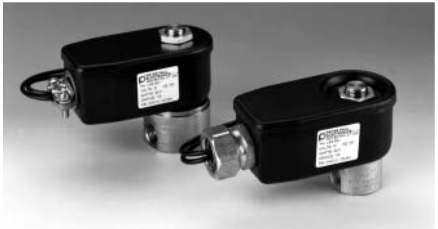
Splice Box option for Peter Paul Series 20 (stainless steel, left) and Series 30 (brass, right) solenoid valves provides space for multiple wiring hookups and an easy access cover for quick and inexpensive field wiring connections directly to the solenoid valve. Splice Boxes shown here with user-provided wire connectors.
