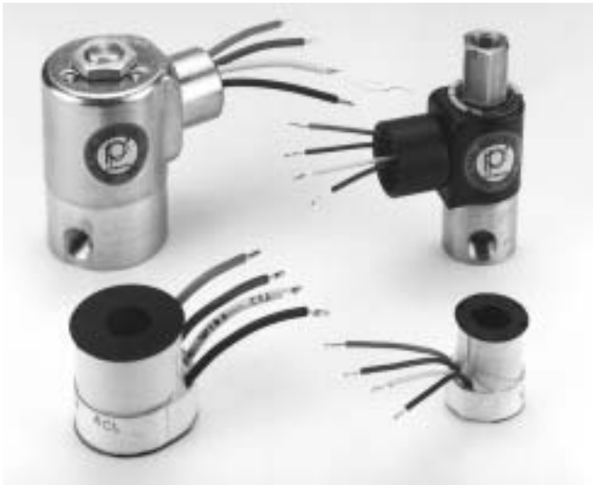
Dual voltage, four-wire coil and completed dual voltage solenoid valve (Series 20, left and Series 50, right) are used when two voltages may be involved in a process, typically 120/240 VAC or 240/480 VAC.
